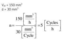
The calculated number of cycles per hour n (5 cycles per hour in this example) is used to determine a working cycle  $T_{WC,S3}.$
