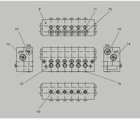
Oil + air metering units are available in two different model designs which differ in terms of available metered quantities of lubricant (see Table 5, Chap. 6.4). The MV20X-20 model design (Fig. 2) is designed for metered quantities between 10 mm<sup>3</sup> and 160 mm<sup>3</sup> (six gradients). The MV50X model design (Fig. 3) supports metered quantities of 2 mm<sup>3</sup> and 6 mm<sup>3</sup>.
